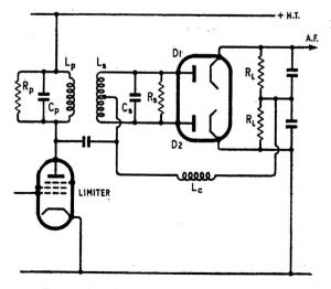
Fig. 1. Basic foster-Seeley discriminator circuit.
