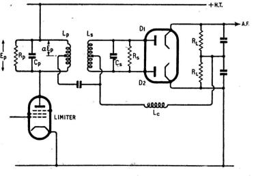
resistor can be connected in parallel with the secondary circuit to achieve this result. Its value can be calculated if it is remembered that the damping imposed on the primary circuit is  $R_L/4\eta$ , whilst that imposed on the secondary circuit is  $R_L/\eta$ . In the example considered above, with equal primary and secondary circuit, the resistance would be  $R_L/3\eta$ .
