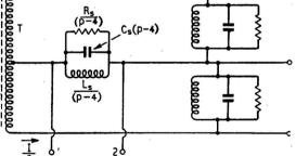
Fig. 3. Equivalent circuit of phase-difference transformer for  $Q_s = \dot{Q}_p$ ;  $p = L_s/L_s$
