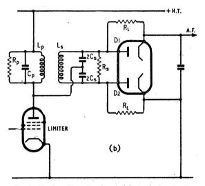
Fig. 8. Further alternative forms of Foster-Seeley circuit, with the secondary circuit centre taps produced by the capacitors.
